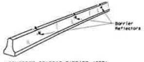
CONCRETE TRAFFIC BARRIER (CTB)
